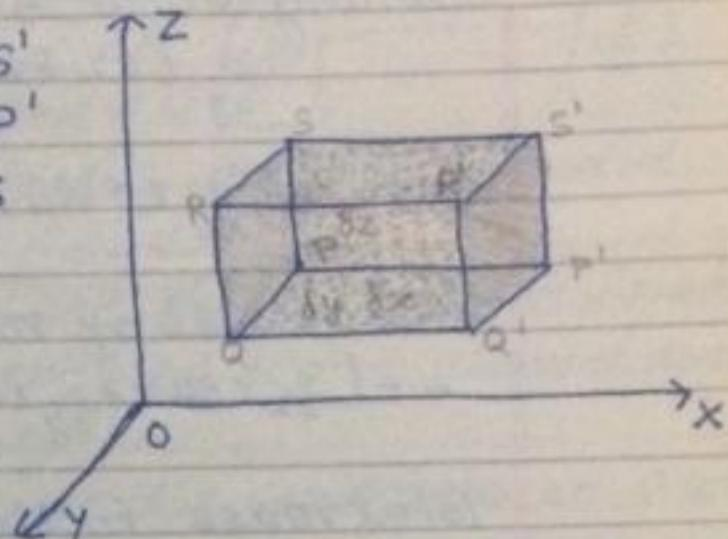
Total accumulation = Excess of the mass that flows in the Parallelepiped over the mass that flows out in time  $\Delta t$
